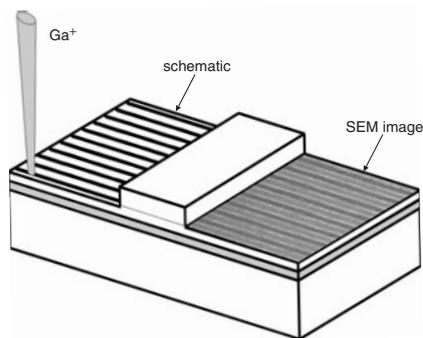
**Fig. 1** Schematic of implantation process and embedded SEM picture of lateral grating with period of 230 nm after etching
