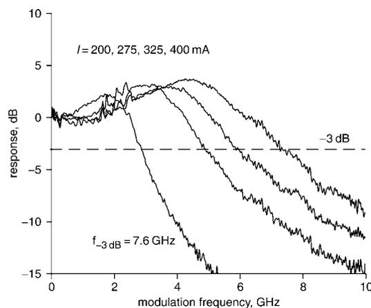
**Fig. 4** Small signal modulation response at four different pulsed (10  $\mu\text{s}$  pulses at duty cycle of 5%) bias levels
