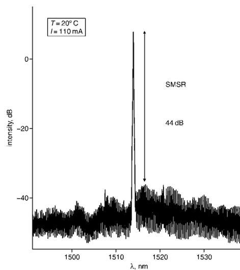
**Fig. 3** Emission spectrum of DFB laser at 20°C with CW drive current of 110 mA
