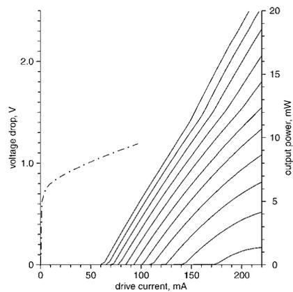
**Fig. 2** P-I curves of 1 mm-long DFB laser with back facet HR coated at different operation temperatures from 15 to 65°C in steps of 5°C
