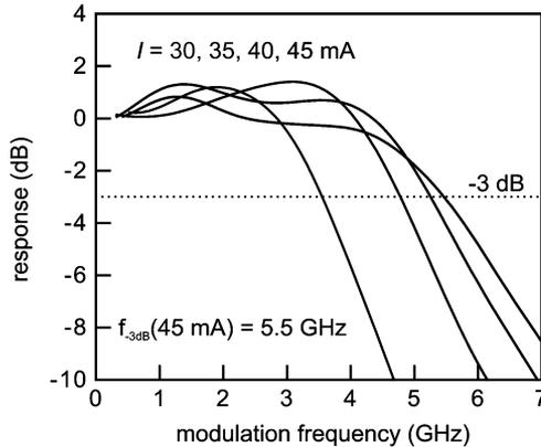
Fig. 5. Small-signal response of a 0.5-mm-long laser at four different CW bias levels.
