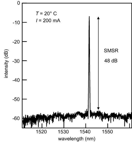
Fig. 3. Emission spectrum of a 2-mm-long DFB laser at 20 °C with CW drive current of 200 mA.
