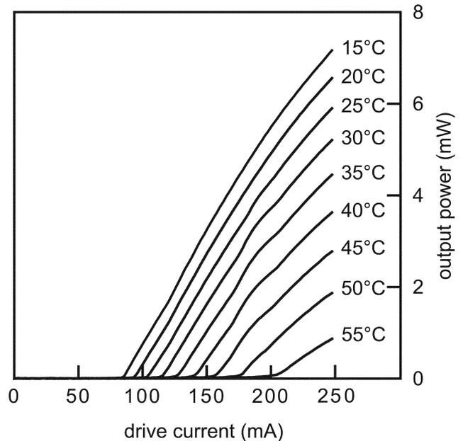
Fig. 4.  $P$ – $I$  curves of a 2-mm-long VG-DFB laser at different CW operation temperatures. The device is as-cleaved.
