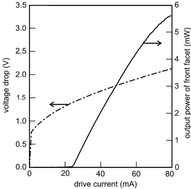
Fig. 2.  $P$ – $I$  and voltage–current curve of a 0.5-mm-long and 2- $\mu$ m-wide VG-DFB laser with back-facet HR-coated. The laser is operated in CW mode at room temperature.
