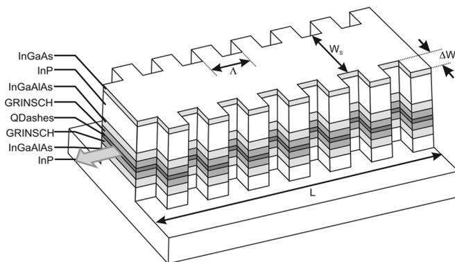
Fig. 1. Schematic structure of a VG-DFB laser.
