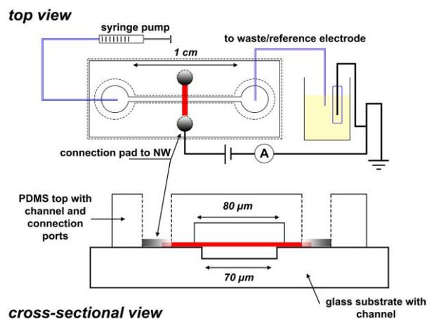
**Figure 2:** Top and cross-sectional schematic of the glass-PDMS device. The NW is depicted as a red stripe. Electrical contact is established with the NW through ports punched in the PDMS.
