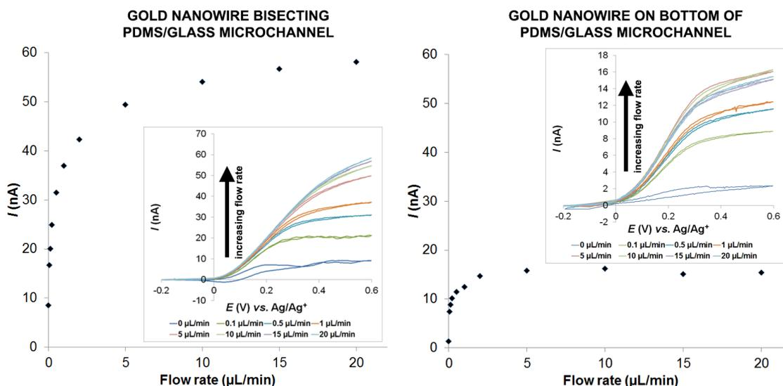
**Figure 3:** Limiting current (at 0.6 V) as a function of the syringe pump flow rate, generated at Au NWs in the center of the flow profile (left) or on the bottom of a microchannel (right). Insets: CVs of single gold NWs, suspended or on a flat substrate, for different flow rates (scan rate of 20 mV/s for all CVs).
