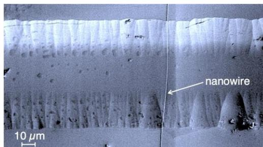
Figure 1: Scanning electron micrograph of a nanoskived gold nanowire suspended over a glass microchannel.
